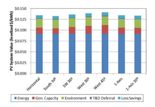
Figure 2: Austin, TX solar photovoltaic value by component and configuration
